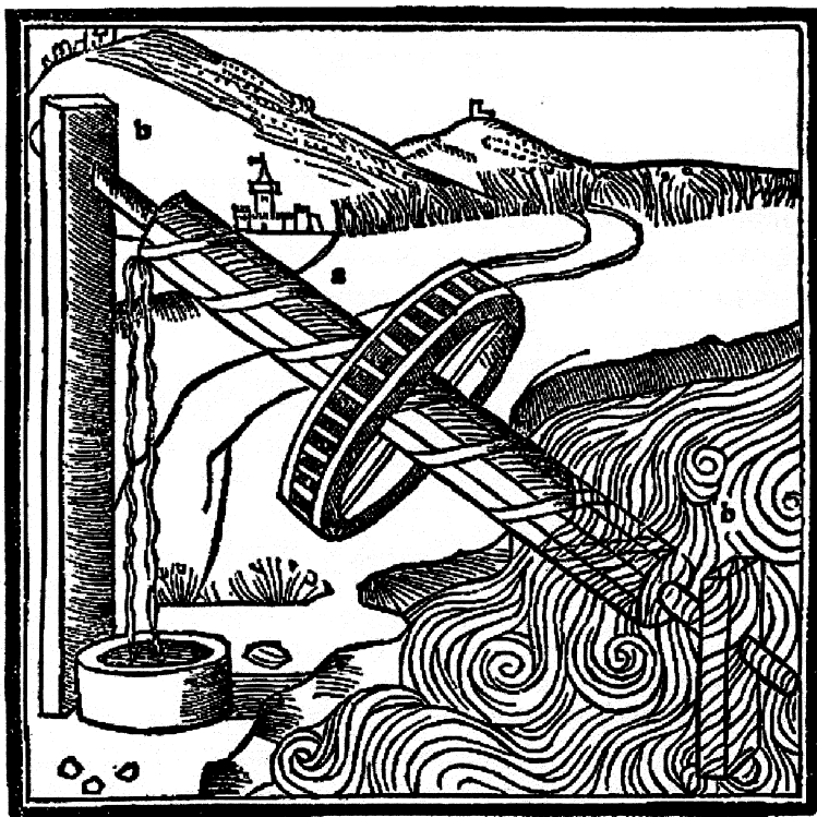
Figure 3. An Archimedean screw mechanism to gain potential energy for water collection from a river.
